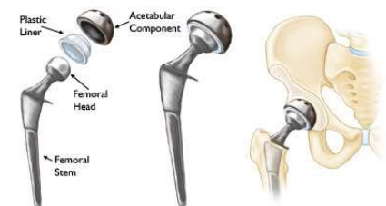
(Left) The individual components of a total hip replacement. (Center) The components merged into an implant. (Right) The implant as it fits into the hip.
